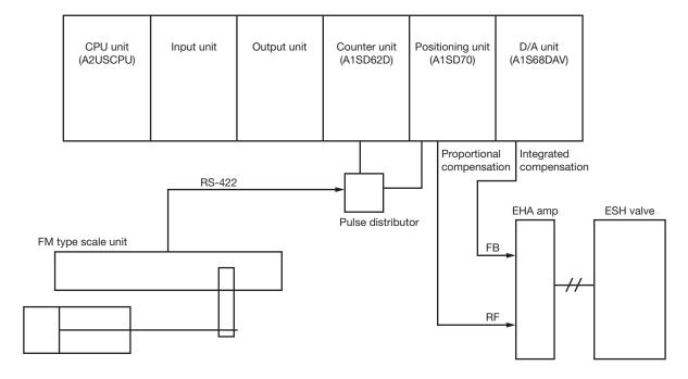
(2) Example Application in ESH-G03, G04, G06 Molding Machine Mold Clamping Circuit
