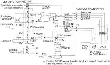
Note) Since G03, G04, and G06 are pilot operation types, there is an LVDT on the main spool, but connection is identical.
